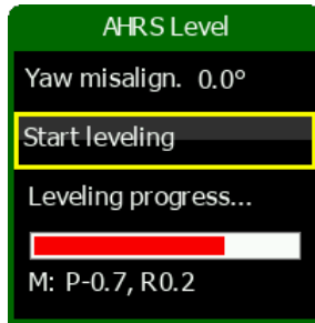
Figure 14: Illustration of AHRS levelling procedure.
