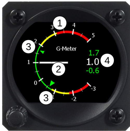
Figure 20: Horis G-Meter screen with markings.
