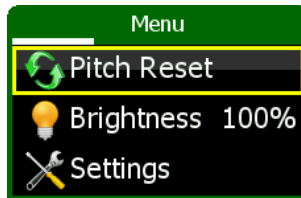
Figure 22: Illustration of Horis main menu. The Pitch Reset option is the default one.
