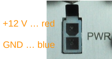
Figure 9: Pins of the power connector.
