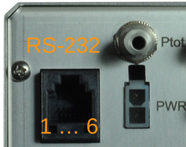
Figure 11: Illustration of the pin out of the RS-232 port.
