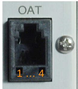
Figure 10: Pins of the OAT connector.
