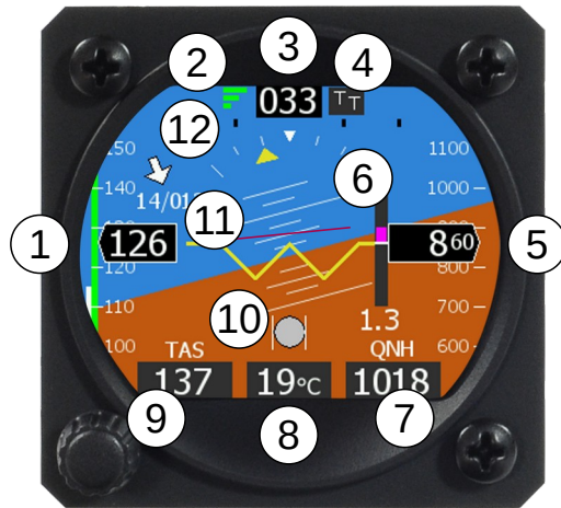
Figure 18: Horis AD-AHRS screen with markings.
