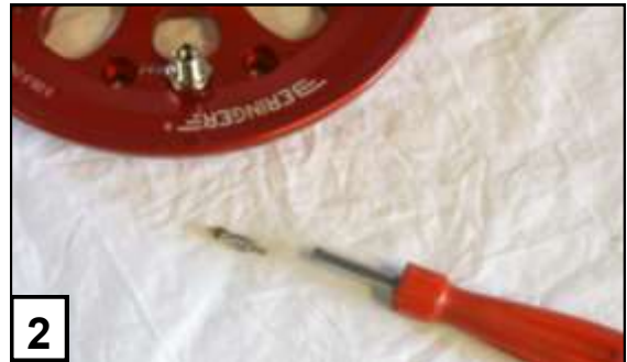
Remove the needle valve with the appropriate tool as detailed above.
