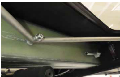
Wing spar joints
