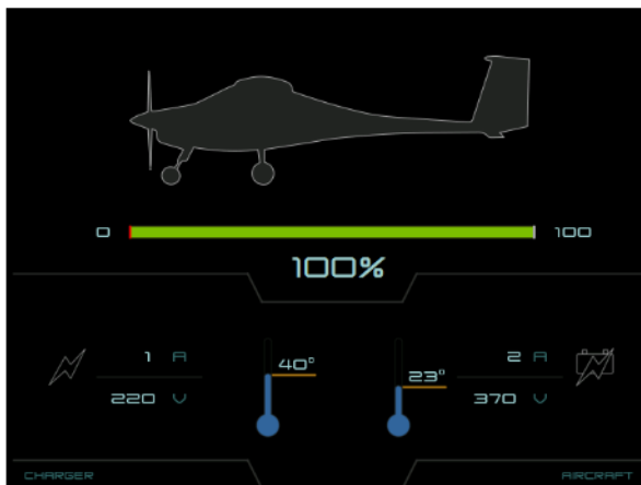
EPSI570C display during charge process - example: charge 100% (completed)
