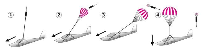
This system is equipped with a parachute canopy, which in most cases is pulled up using a solid fuel rocket engine. The parachute canopy is connected to the aircraft by a suspension system (steel ropes/straps).
