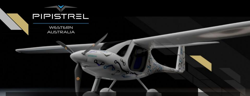
Alpha Electro is a 2-seat electric trainer with performance which is tailored to the needs of flight schools. It has short take-off distance, powerful 1000+ fpm climb capability and an endurance of one hour plus a 30-minute reserve. The Alpha Electro is optimized for traffic-pattern operations, where up to 13% of energy is recuperated on every approach, increasing operations range and at the same time enabling short-field landings.
