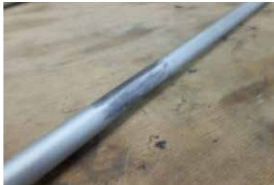
Figure 27-010 Horizontal elevator pushrod surface discoloration
