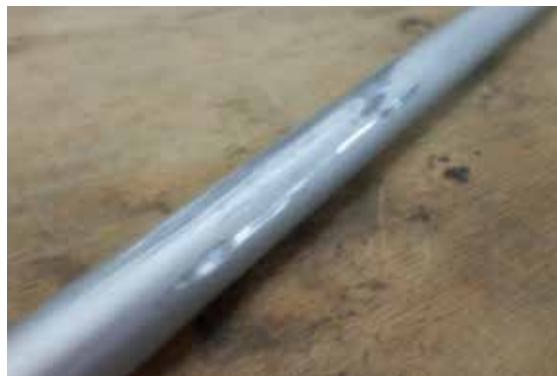
Figure 27-011 Horizontal elevator pushrod surface gouges
