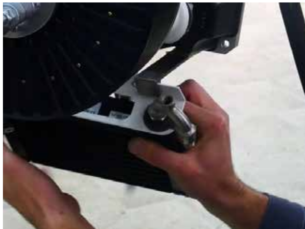
Figure 75-002 Correct cooler outlet positioning
