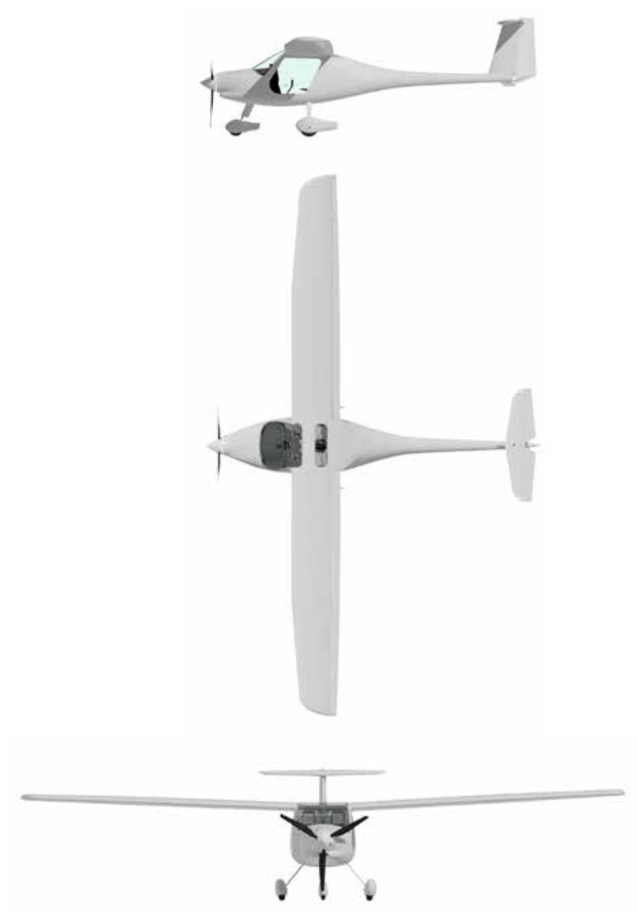
Figure 06-001 ALPHA Electro three view drawing
