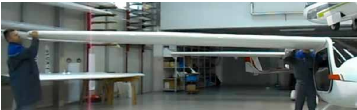
Figure 57-001 Support the wings
