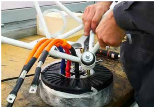
Figure 72-002 Sliding motor mount
