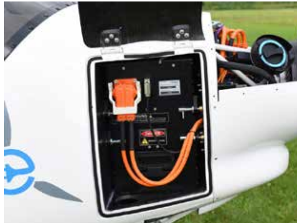
Figure 24-002 Installed fore battery box
