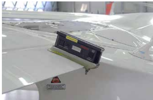
Figure 27-0017 Flaperon deflection angle adjustment
