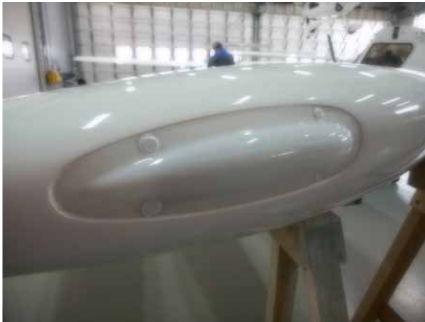
Figure 33-001 NAV/STROBE light installation
