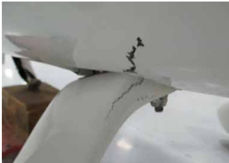
Figure 53-001 Example of fuselage main frame damage
