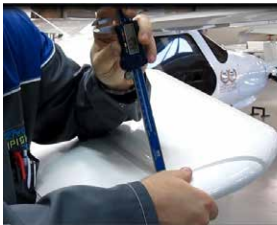
Figure 27-009 Elevator radial free play check
