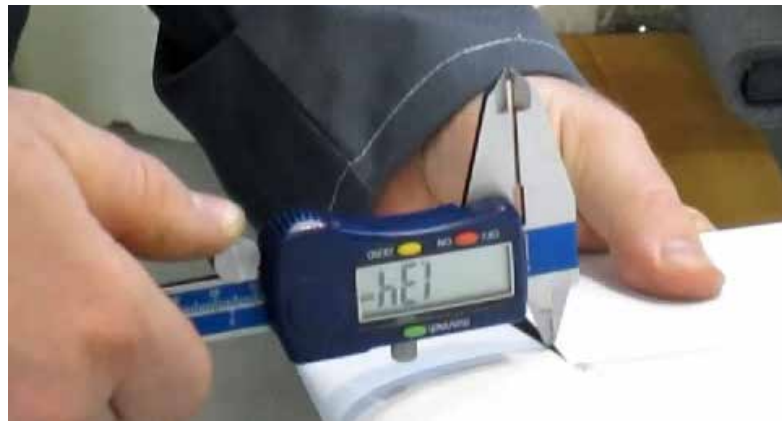
Figure 27-014 Flaperon axial free play check
