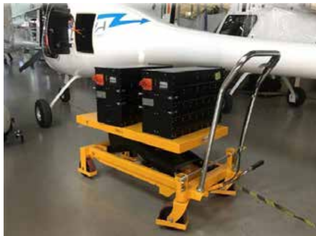
Figure 24-001 Fore and aft battery boxes
