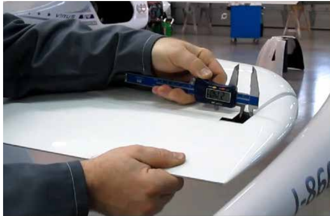
Figure 27-008 Elevator axial free play check
