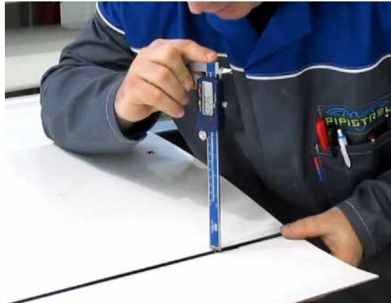
Figure 27-015 Flaperon radial free play check
