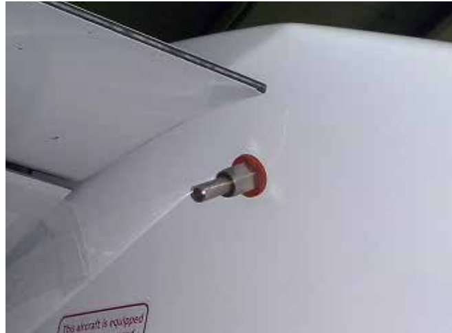
Figure 34-002 OAT sensor installation
