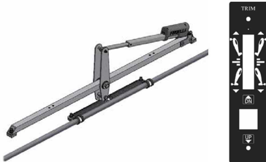
Figure 27-007 Elevator trim system and cockpit switch/display
