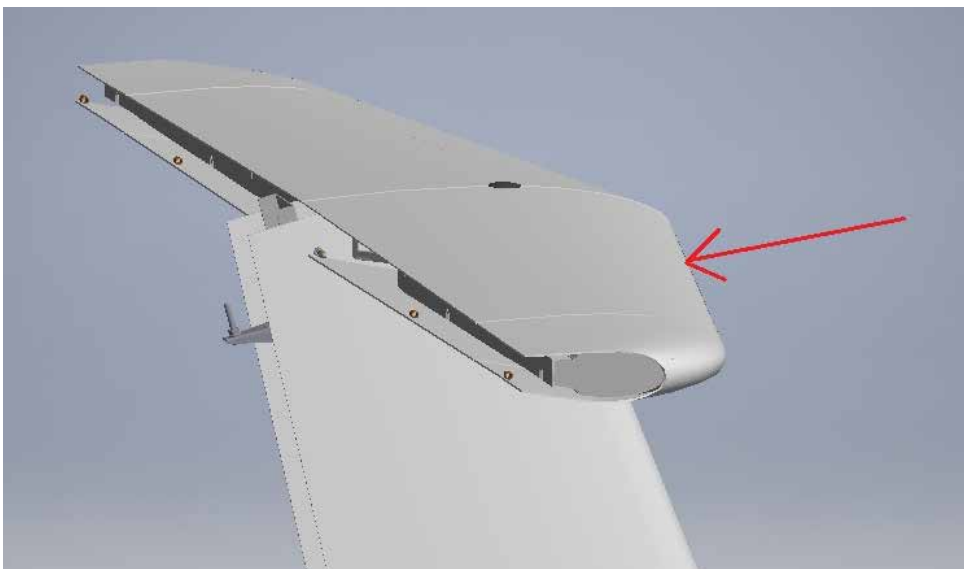
Figure 51-004 Horizontal stabilizer leading edge bonding line
