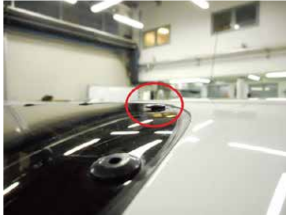
Figure 56-004 Example of loosened window rivet
