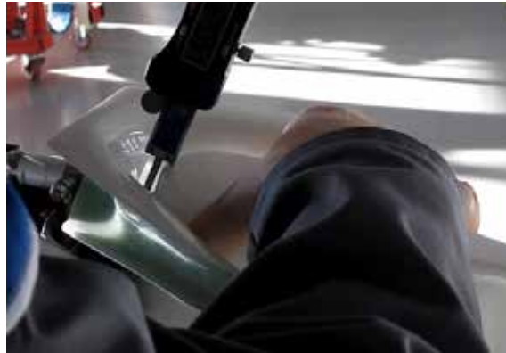
Figure 27-005 Rudder axial free play check
