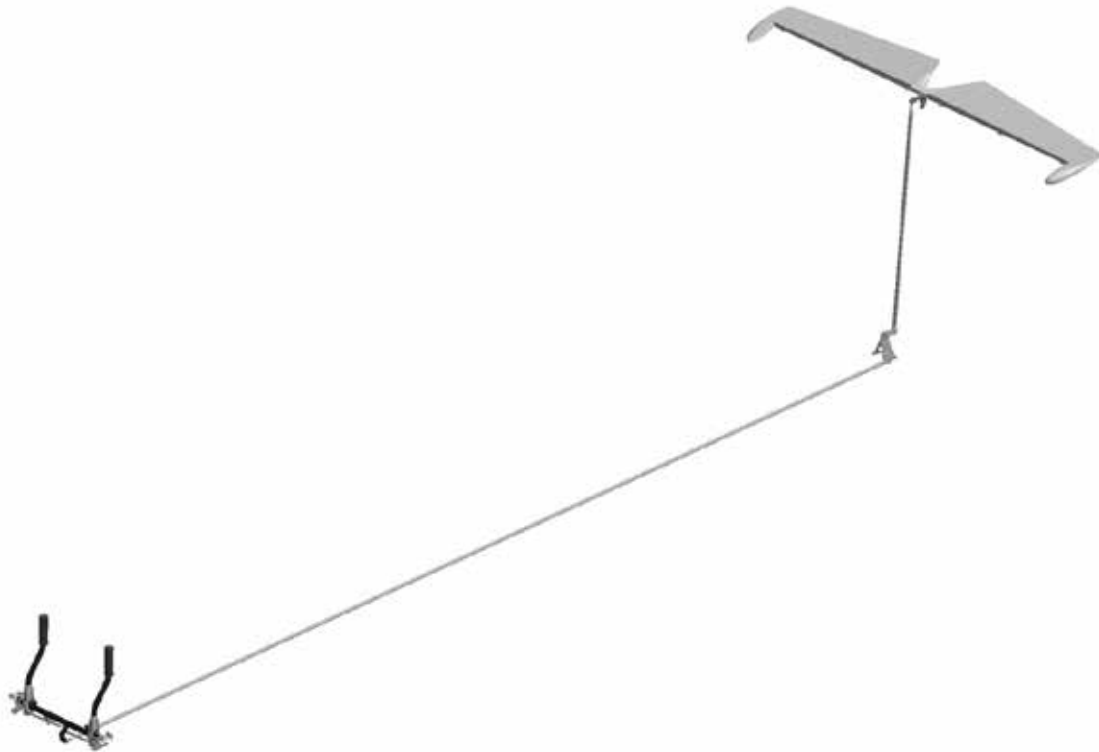
Figure 27-006 Elevator control system
