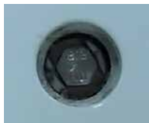
Figure 55-002 Attachment bolt assembly head orientation
