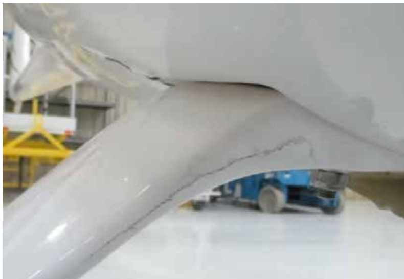
Figure 32-003 Example of a damaged MLG strut
