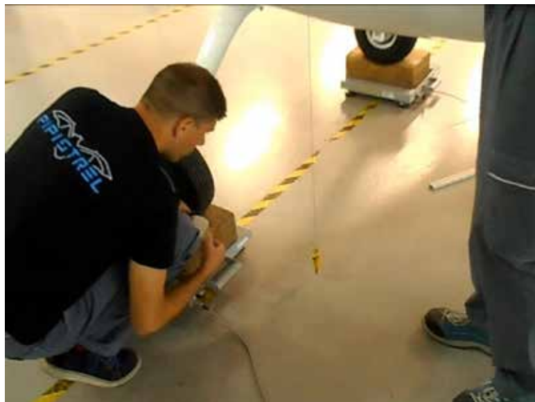
Figure 08-002 Plumb bob from wing leading edge
