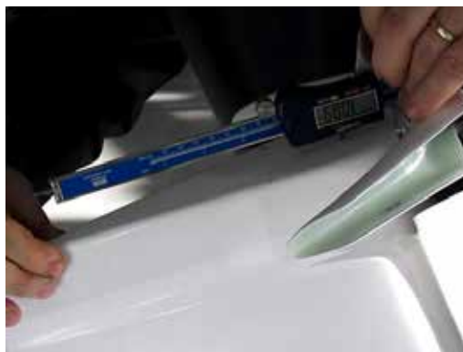
Figure 27-004 Rudder radial free play check
