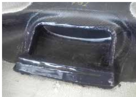
Figure 71-001 Baffling between lower cowling and cooler
