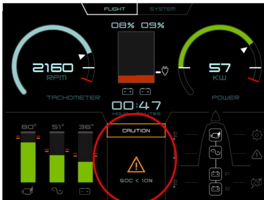
EPSI570 screen area displaying warning and caution messages
