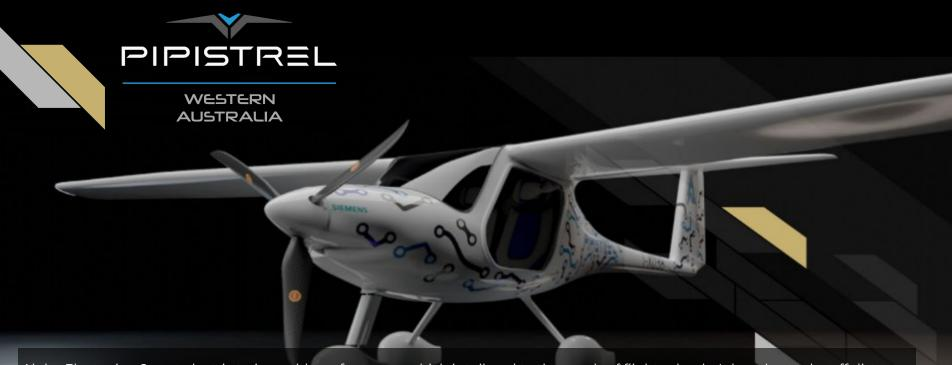
Alpha Electro is a 2-seat electric trainer with performance which is tailored to the needs of flight schools. It has short take-off distance, powerful 1000+ fpm climb capability and an endurance of one hour plus a 30-minute reserve. The Alpha Electro is optimized for traffic-pattern operations.
